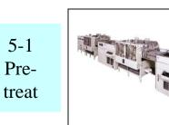
Pumice Line : Clean foreign material from board surface and roughen board surface to increase adhesion to dry film
