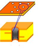
resin smear on hole wall
