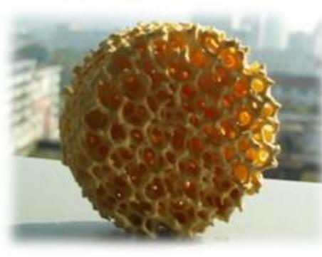
AGS-Industrial Zirconia Ceramic Foam Filters (CFF-ZR) is available in all common sizes in the range of 40x40x20mm up to 150x150x30mm. Round filters are available from D40x20mm up to D150x30mm. Although PPI 10 is the porosity most commonly used for steel casting, finer porosities up to PPI 60 are available on request. Custom-made cut-to-size filters are also possible.
